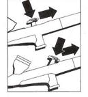
press down for air, pull back for paint. The further the lever is pressed down, the stronger the air force, the further the lever is pulled back, the greater the amount of paint. The balancing act of blending the right amount of air and paint comes with experience.
